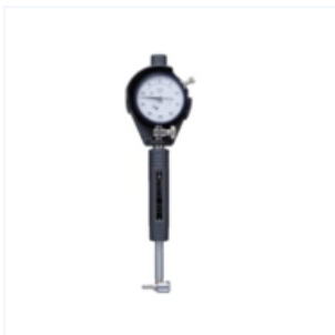
Mitutoyo CG-250AX Standard Cylinder Gauging Tool 220 mm
